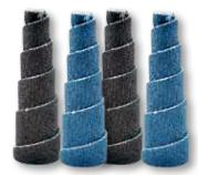
Multi-layered abrasive tool which renews its cutting surface. Cartridge rolls are ideal for welds and mark removal, edge breaking, sanding of inside diameters. This tool reaches into corners, where larger diameter tools cannot work.
