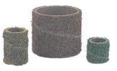
Spiral bands are made of high quality abrasive cloth rolled and fixed on a tear-resistant fabric. This spiral design ensures a smooth even cutting action. Spiral bands are ideally suited for grinding and finishing edges, profiles, welded joints, opening, etc.
