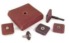
Aluminum oxide abrasive square pads are used for blending welds, interior diameter finishing and deburring of flat surfaces. Can be made with other minerals. Standard with threaded eyelet.
