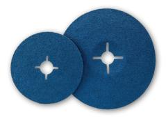
Fiber discs have a tough vulcanized fiber backing. Use for heavy duty grinding and high stock removal on metal, steel and cast iron. Also available in aluminum oxide, ceramic and zirconium.
